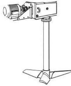
Fig. 7b. Impeller and motor for a mixing tank
