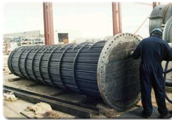
HE 1-2 ( 1 pass in shell, 2 passes in tube)
